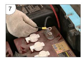
5. The unplugged charging cable is no longer in use, wrap it with insulating tape.
