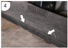
5. Drilling must be be 90° vertically.
