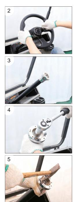
8. Remove the steering wheel mounting adapter.
