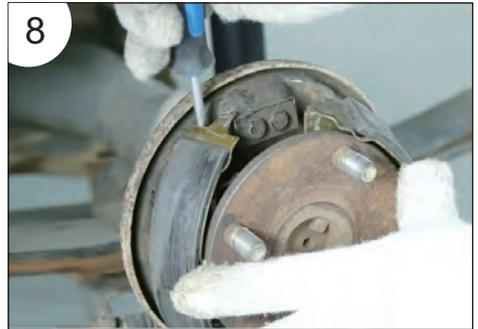
11. Install a new brake shoe and the brake spring; (Note: Both the brake shoe and the brake spring must be installed in the correct position as shown in the picture. )
