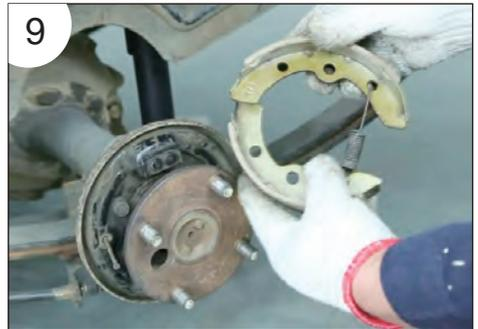
12. Install the shoe retainer with the long flat nose pliers.
