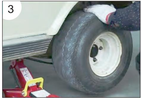
6. Remove the front wheel; then put the wheel under the chassis (in case the jack accidentally leans or slips down)
