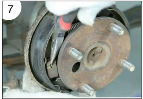
10. Remove the brake shoe with the slotted screwdriver.
