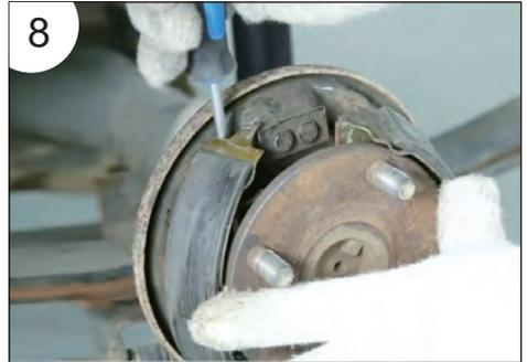
11. Install a new brake shoe and the brake spring; (Note: Both the brake shoe and the brake spring must be installed in the correct position as shown in the picture. )
