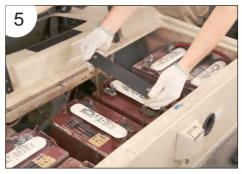
Put the the battery hold down and J bolts back in place and tighten the locknuts with a 9/16-inch (14mm) socket.
